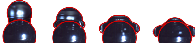
FIGURE 1. Snapshots of drop impact onto a solid sphere, in which a water drop of D = 2.22 mm hits a steel sphere of 3 mm in diameter at an impact velocity of U_0 = 0.74 m s -1 . The advancing contact angle \theta_A = 95^\circ in experiments. Numerical results at We = 16.8 , Re = 1638 , \theta = 95^\circ and \lambda_r = 1.35 (solid curves) are superimposed on the experimental results at dimensionless times tU_0/D = 0.2, 0.45, 0.9 and 1.35 (from left to right).
