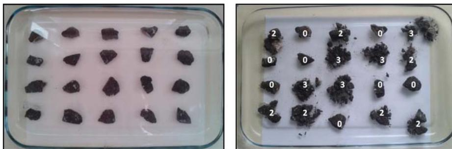
FIG. 6. Sample M1 in slake test. Start of test (left), end of test (right). Averaged index of deterioration = 1.45.
