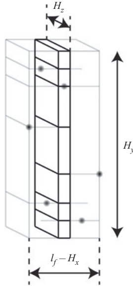
FIGURE 7. Sketch of a very thin slice. All fractures with their centres in [H_x - l_f/2, l_f/2] \times [0, H_y] intersect with both the left and right boundaries.
