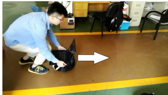
Fig. 11. Kidnapping manually. The robot is in the current position before kidnapping, and it is moved manually along the arrow.
