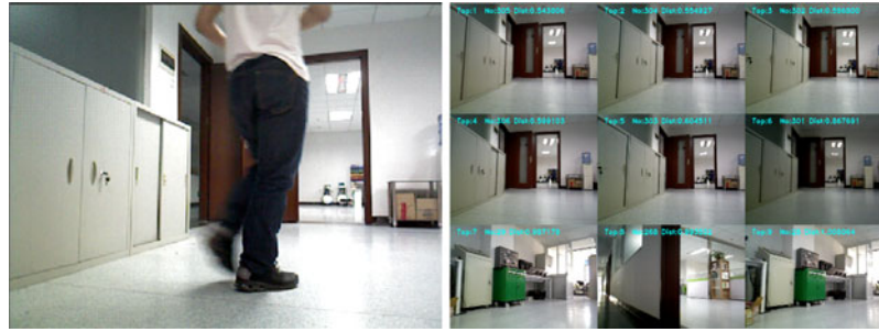
Fig. 13. Result of image matching. The left figure is the current observation and the right figure is the result. The top six matching results are correct, even there is a new object in the query image.
