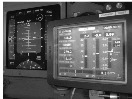
LADS as installed on a flight deck, next to Primary Flight Display
