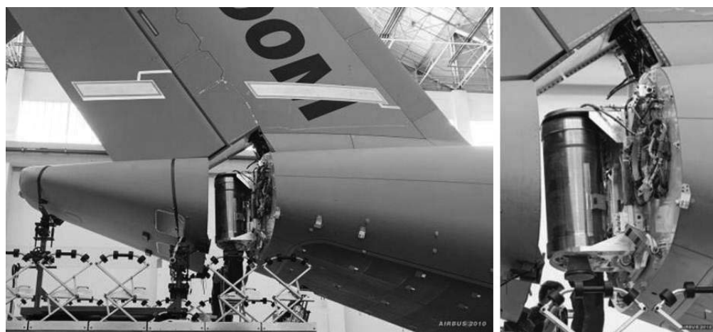
Figure 16. Tail booster installation.
