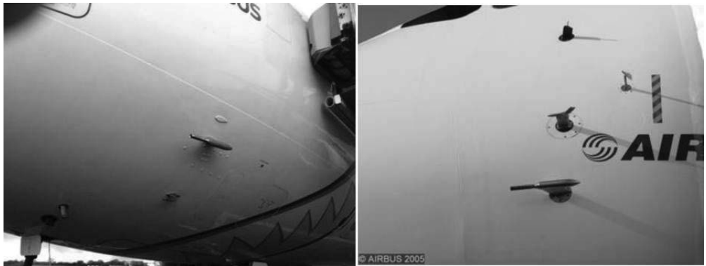
Figure 12. Flight test pitot installation.
