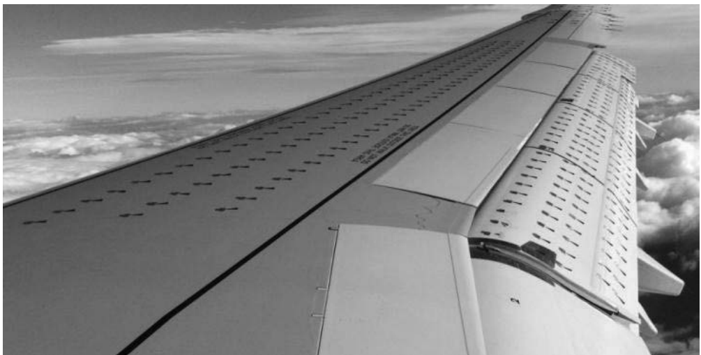
Figure 13. Flow cone installation.
