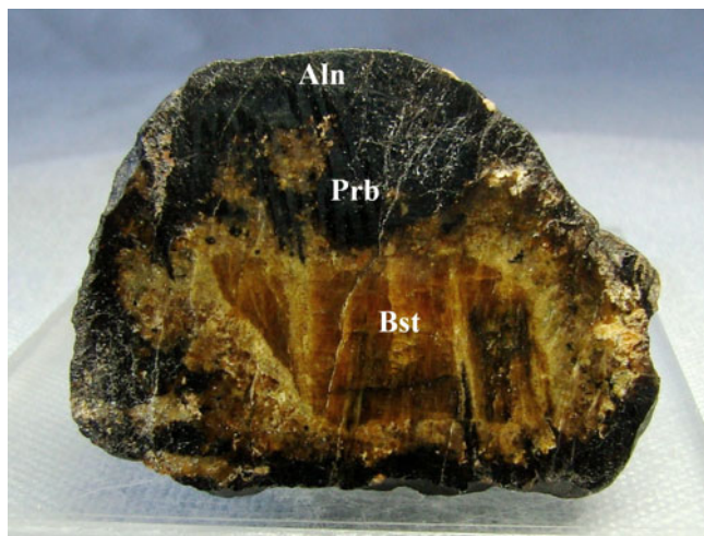
Fig. 3. Cut and polished nodule showing typical ovoid structure: orange-yellow core of bastnäsite (Bst), black middle zone of perbøeite/ferriperbøeite (Prb) and black rim of allanite/ferriallanite (Aln). Size of the sample: 2 cm × 1.7 cm. Photo: A.M. Kuznetsov, specimen no. ML 59-2.
