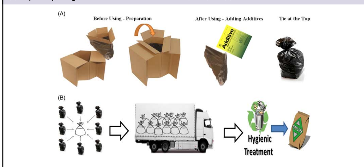
(A) Steps for Operating the Waterless Portable Private Toilet (WPPT) and (B) Collection and Treatment of WPPT Waste.
