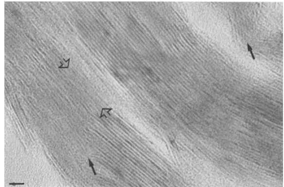
Figure 7. Lattice fringe image with 2 nm spacing throughout. The particles have been bent, possibly during compaction (black arrows). Cross fringes (between the open arrows) indicate lattice continuity. The sample is from 2222.6 m and was prepared by ultramicrotomy without fixation of expandable layers. Scale bar = 5 nm.
