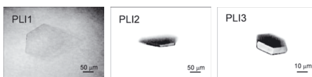
Fig. 1. Typical PLIs observed in the EPICA-DML ice core. All PLIs shown here are from the 1474 m depth sample. PLI1 is the thinnest (~1–2 \mu\text{m} thick), while PLI2 and PLI3 are no thicker than 5 \mu\text{m} .
