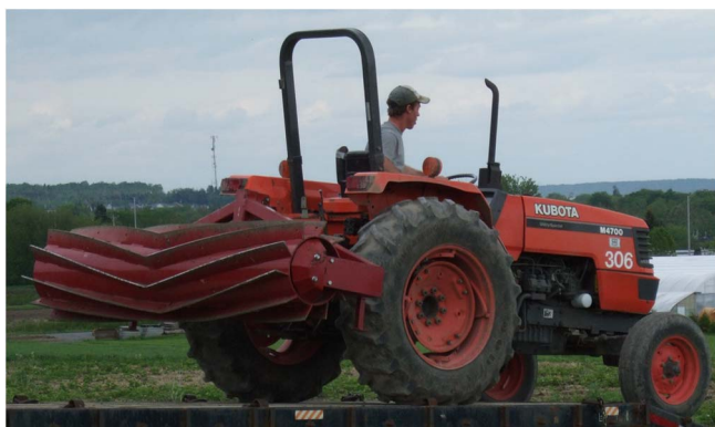
Figure 2. Roller-crimper used at the Laval University Agronomic Station. The roller-crimper is 2.4 m long by 40 cm diam with 20 cm separated blades arranged in chevron pattern and weighs 920 kg when filled with water (I&J Manufacturing, Gordonville, PA).
