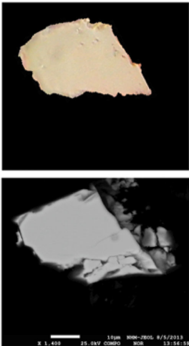
Fig. 3. Secondary electron image of an agmantinite grain and its optical image under crossed polars. Scale bar = 10 \mu\text{m} .
