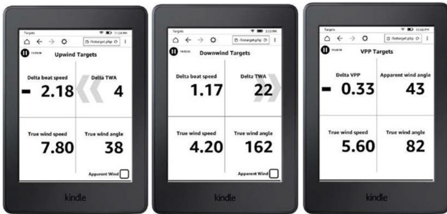
Figure 4. (Left) The upwind target screen shows the error of the boat speed (too slow by 2.18 knots), the error of the true wind angle (4 degrees too close to the wind), the actual speed and angle of the true wind. The cues (background arrows) suggest steering to the left, away from the wind. (Centre) Similar data, but when sailing downwind. (Right) The wind-abeam target screen, that shows the speed error (too slow by 0.33 knots) along the current course, not in the direction of the wind as before.
