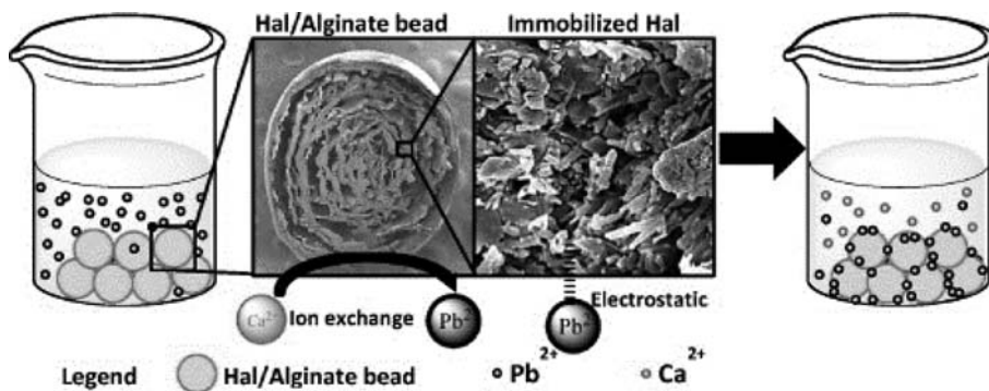
FIG. 4. Pb^{2+} removal/adsorption by halloysite/alginate nanocomposite beads (from Chiew et al. , 2016; reproduced here with the permission of Elsevier).
