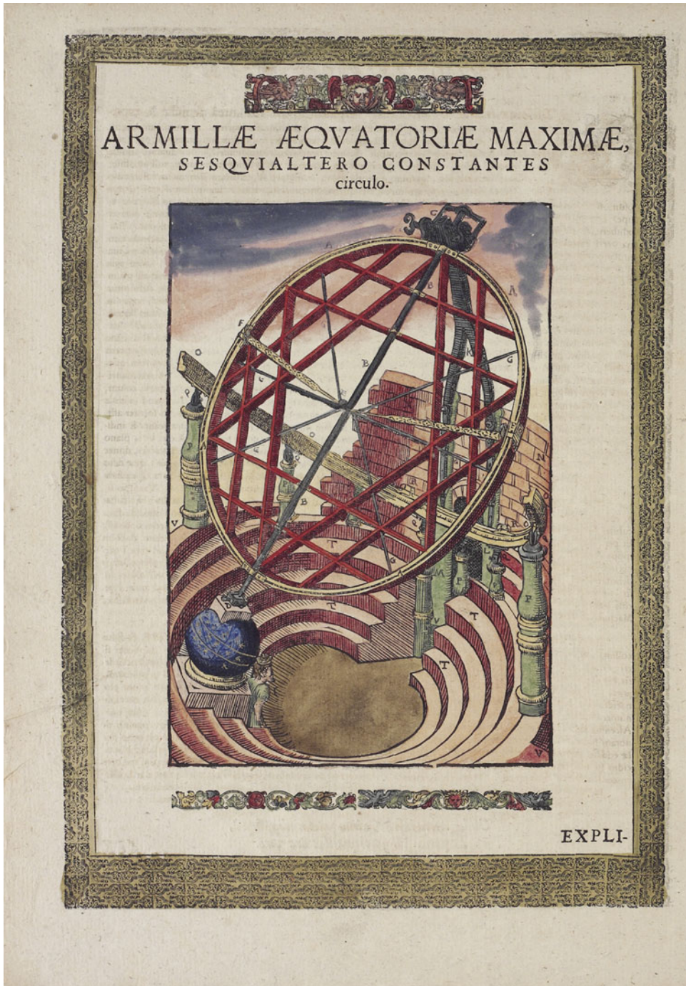
Figure 9. Armillae aequatoriae maximae, sesquialtero constantes circulo (Great equatorial armillary instrument with one complete circle and one semicircle). Woodblock engraving on paper, water-soluble paint and gilt.
