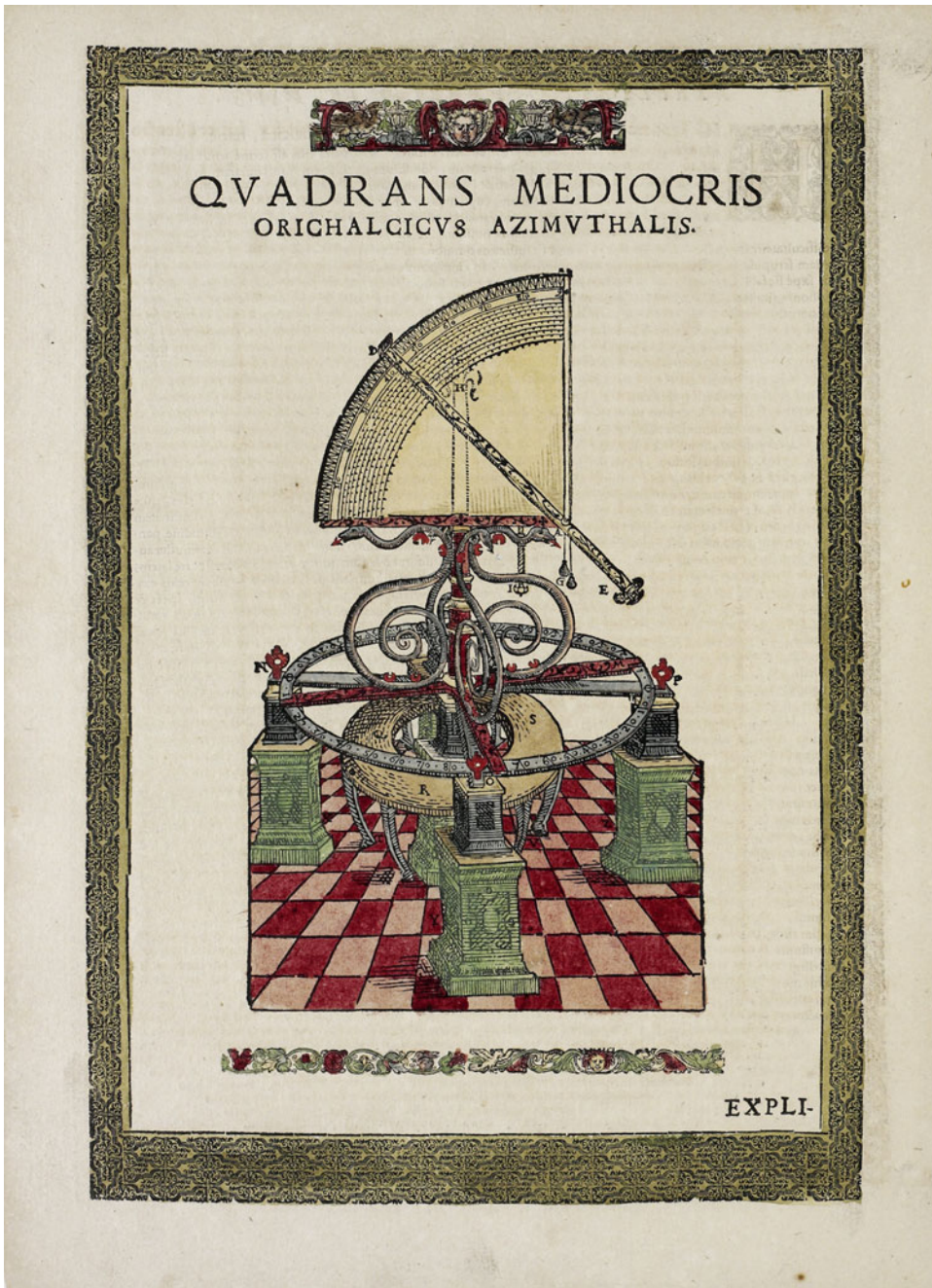
Figure 10. Quadrans mediocris orichalcicus azimuthalis (Medium sized azimuth quadrant of brass). Woodblock engraving on paper, water soluble paint and gilt.
