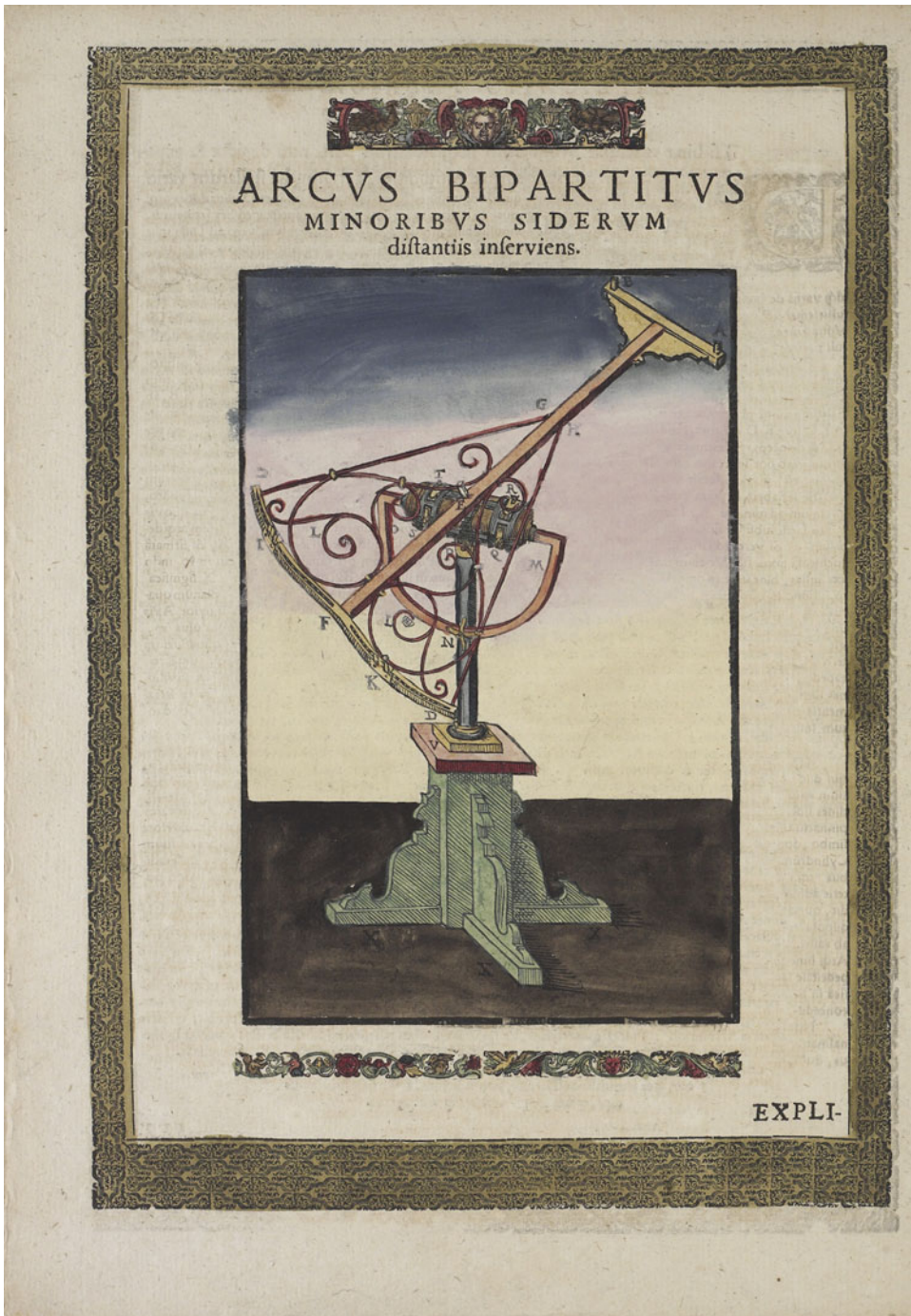
Figure 4. Arcus bipartitus minoribus siderum distantis inserviens (Bipartite arc for measuring angular distances). Woodblock engraving on paper, water soluble paint and gilt.
