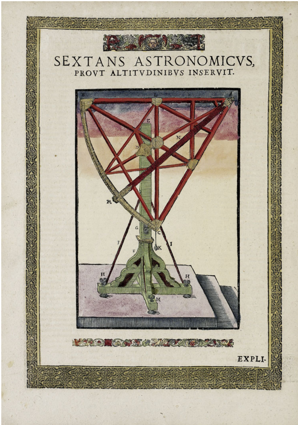
Figure 5. Sextans astronomicus, prout altitudinibus inseruit (Astronomical sextant for measuring altitudes). Woodblock engraving on paper, water-soluble paint and gilt.
