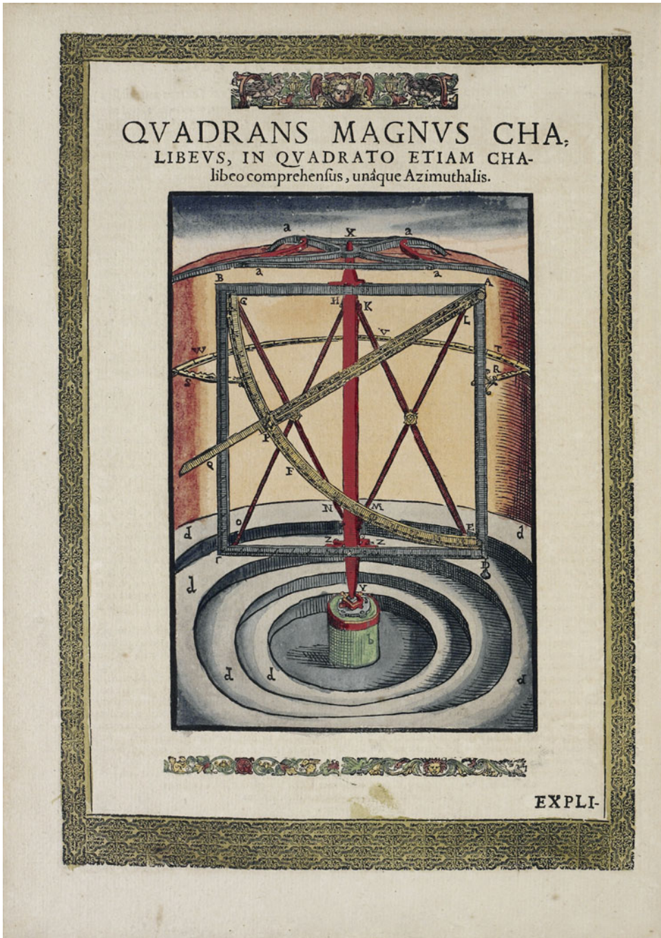
Figure 7. Quadrans magnus chalibeus, in quadrato etiam chalibeo comprehensus, unaque azimuthalis (Great steel quadrant, inscribed in a square, also of steel, and revolving in azimuth). Woodblock engraving on paper, water-soluble paint and gilt.
