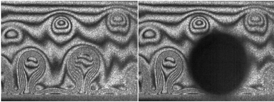
FIGURE 15. Spontaneous bursting at the foot of a flat water film (interference fringes visualized by a monomode argon laser at 488 nm). Nucleation is seen to occur around a convection cell: the paradigm situation in the bursting of bubbles. Image height is 3 mm and time lapse between the two images is 1/3000 s. The film receding velocity is V = 2.8 \text{ m s}^{-1} corresponding to a thickness h = 20 \text{ }\mu\text{m} .
