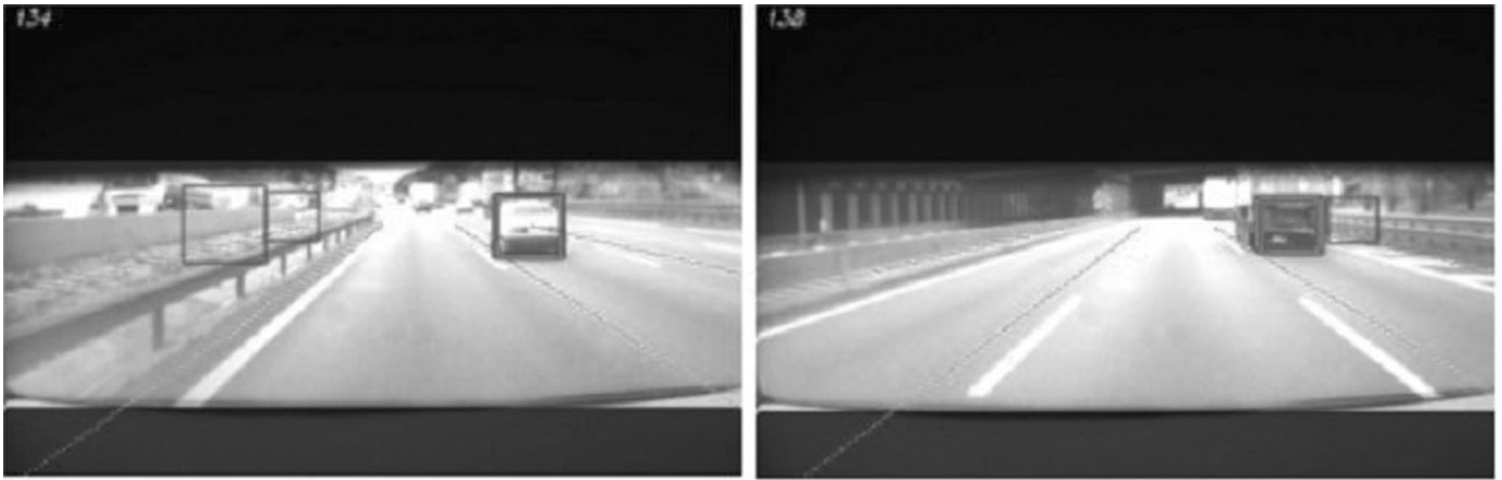
Fig. 10. Examples of initial candidates detected by the attention mechanism (vehicles and non-vehicles).
