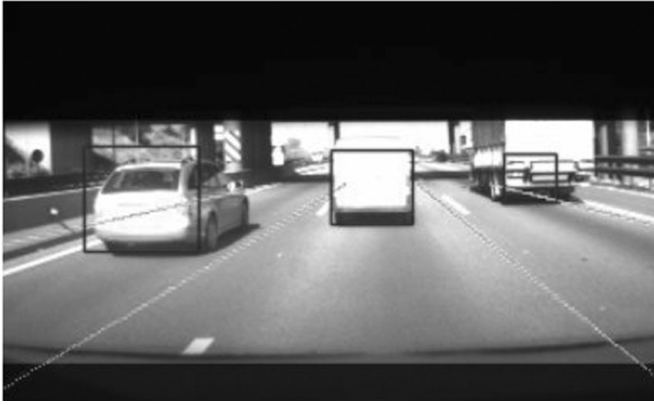
Fig. 21. SVM-based classification stage can be divided in three modulus, one for each lane.
