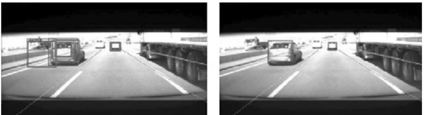
Fig. 9. Candidate overlapping removal in the attention mechanism: original candidates (left); result after overlapping removal (right).
