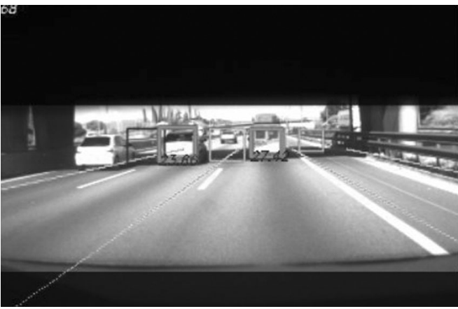
Fig. 22. Example of false vehicle detection.
