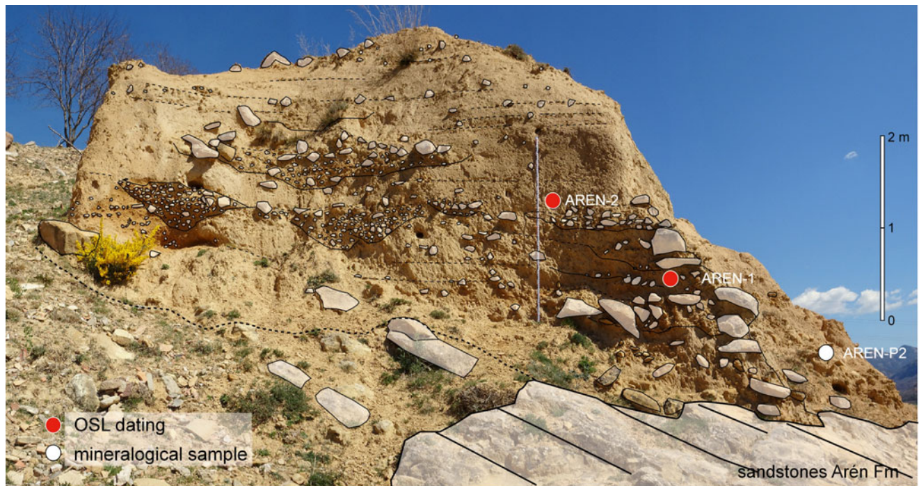
Figure 7. Photoschematic of the stratigraphic units in the sandy deposit close to Arén, showing the sampled points for OSL dating (AREN-1, AREN-2) and the sample point for mineralogical analysis (AREN-P2). Thin dashed line = bedding planes; Thick dashed line = presumed contact with Arén Formation; thin solid lines = channel base; thick solid lines = Arén Formation contact; larger clasts are outlined by thin solid lines.
