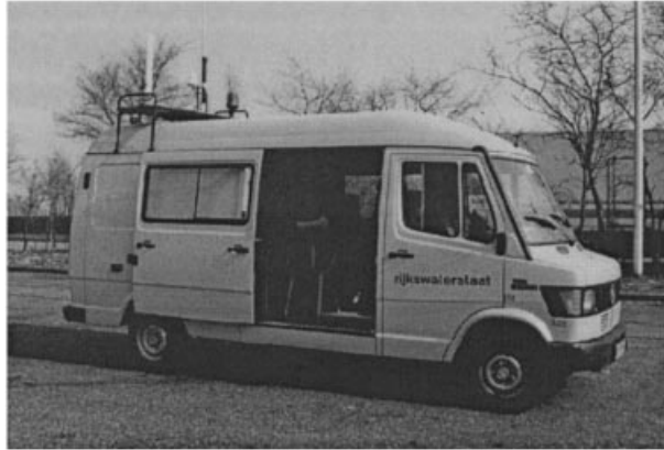
Figure 7. Measurement Van of the Dutch Survey Department.
