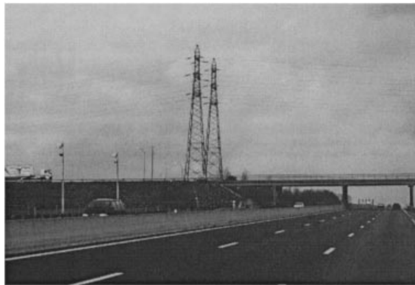
Figure 8. Example of a Difficult Environment for Loran-C Reception.
