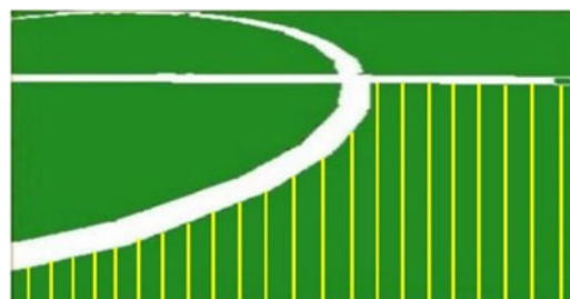
Figure 7 A total of 320 scan lines are applied to calculate the distance from the first white-line pixel to the bottom
