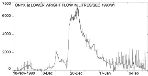
Fig. 88. 1990–1991. Onyx at Lower Wright instantaneous discharge record.
