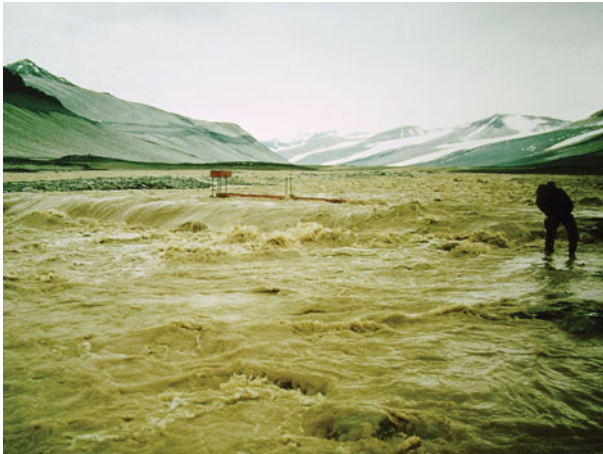
Fig. 81. 1986–1987. Upstream view of the weir and water level recorder during the January flood. Note the stream in the background flowing in a separate channel (Photo. C. Lynch).
