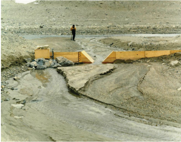
Fig. 56. 1982–1983. The sediment-loaded Clark stream flume with surface follower recording instrument.
