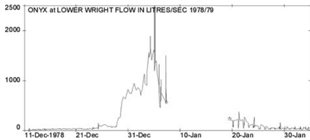
Fig. 34. 1978–1979. Onyx at Lower Wright instantaneous discharge record.
