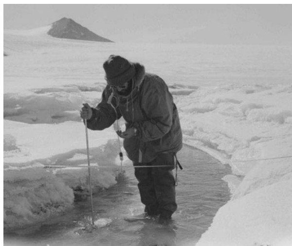
Fig. 43. 1979–1980. Gauging flow in an ice channel, Lower Wright Glacier.
