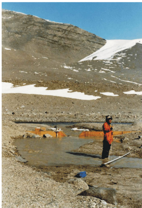
Fig. 94. 1983–1984. Making a flow gauging at the Clark flume.
