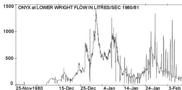
Fig. 44. 1980–1981. Onyx at Lower Wright instantaneous discharge record.
