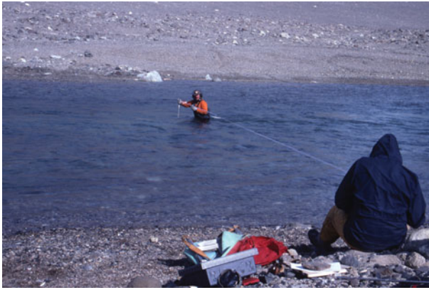
Fig. 73. 1985–1986. Mason and Potter flow gauging at a high stage in the Lower Wright Reach.
