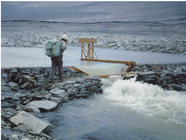
Fig. 11. 1970–1971. The first of many overtopping events at the weir which occurs at flow of approximately 2 cumecs.
