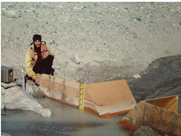
Fig. 61. 1983–1984. Robertson attending to the Clark Flume surface follower recorder. Note the dirty water—the main source of sediment in the Onyx River.
