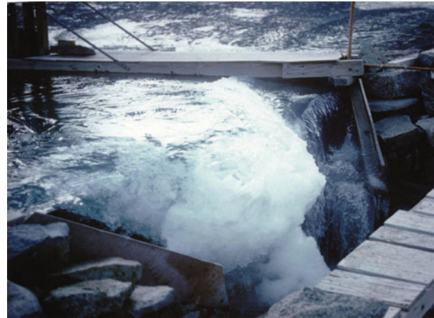
Fig. 71. 1984–1985. A severe case of icing of the Onyx weir notch in 1984–1985. In this case the ice growth has expanded to fill and close the entire V-notch to produce an erroneous spike on the stage record.
