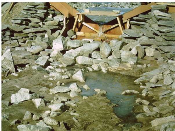
Fig. 8. 1969–1970. The first flow of the season passing through the V- notch of the measuring weir across the Onyx near Vanda Station. It was hoped that the 'hood' over the notch would reflect radiation downward to melt any ice accretion.
