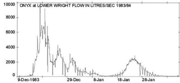
Fig. 57. 1983–1984. Onyx at Lower Wright instantaneous discharge record.
