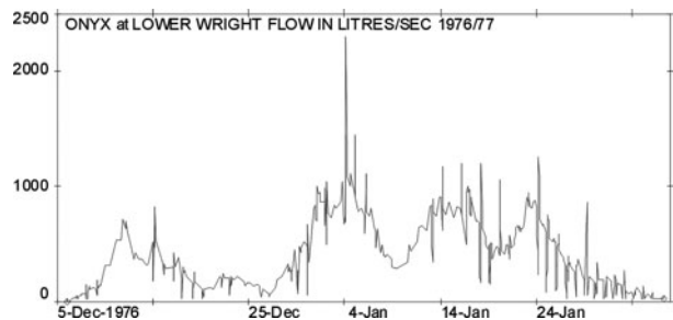
Fig. 30. 1976–1977. Onyx at Lower Wright instantaneous discharge record.
