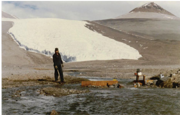
Fig. 65. 1984–1985. Bartley flume damaged by an overtopping flow.
