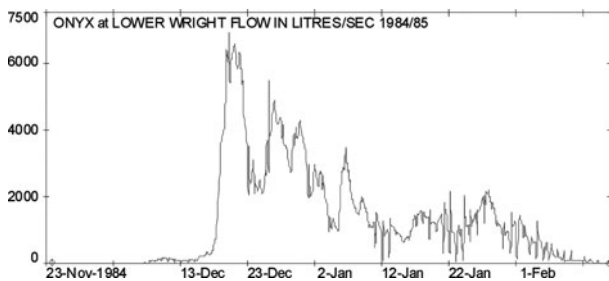
Fig. 69. 1984–1985. Onyx at Lower Wright instantaneous discharge record.
