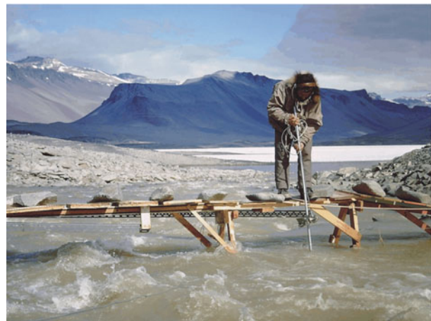
Fig. 13. 1970–1971. Baker measuring the discharge on the flood gauging bridge using a bucket-type current meter. Lake Vanda in background.
