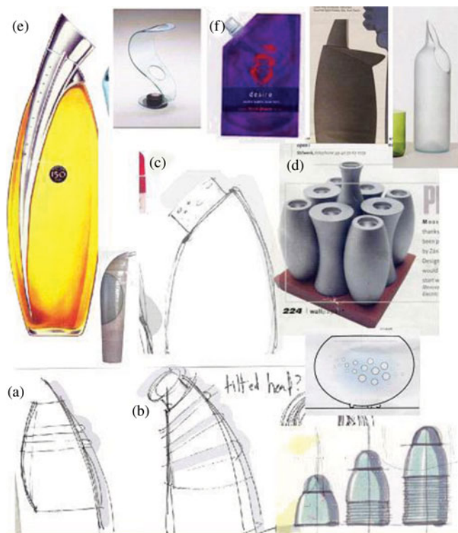
Fig. 11. Moodboard for product design showing multiple sketches of the object and the sources of inspiration for it. Although we do not know the role for which the rough sketches were originally drawn, they give a good impression of an idea generation sketch in product design. [A color version of this figure can be viewed online at http://journals.cambridge.org/aie ]
