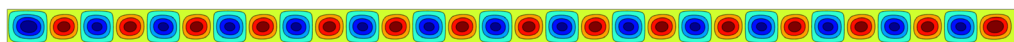
Figure 9. Counter-rotating convection rolls generated by Rayleigh–Bénard convection. This flow field is used to study fronts propagating through a cellular flow field. Colour contours are of the streamfunction, where red indicates counter-clockwise rotation and blue indicates clockwise rotation. The characteristic fluid velocity is U = 11.29 . Simulation parameters: \Gamma = 30 , Ra_T = 3000 .
