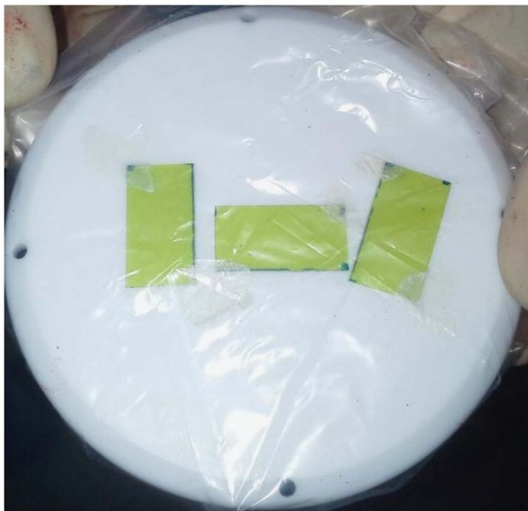
Figure 1. Three pieces of EBT-2 film cut into 1 × 1.5 and on top of protection disk and wrapped by sterile envelope.
