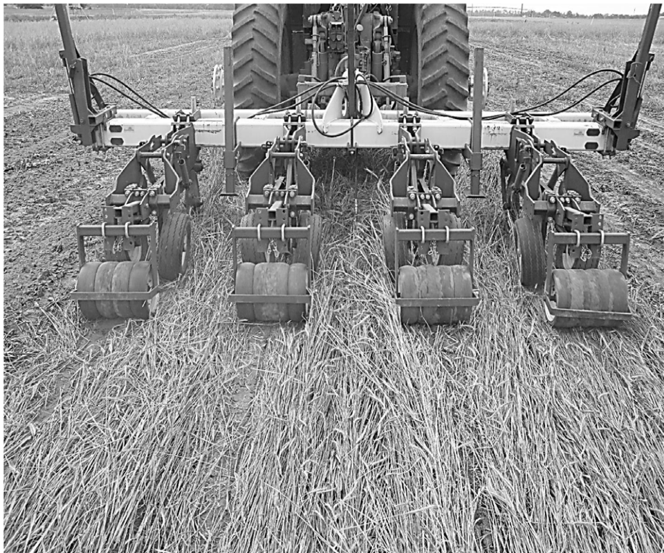
Figure 2. A narrow residue disturbance (<5 cm) 4-row 3-m KMC® Generation 2 subsoiler/leveler implement (Kelly Manufacturing Company) equipped with two pneumatic tires and hard rubber rollers.
