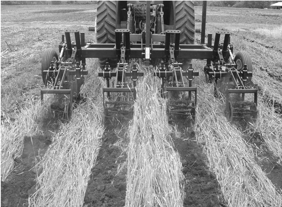
Figure 1. A wide residue disturbance (30 cm), 4-row 3-m KMC® Generation 1, 16 Series rip/strip till implement (Kelly Manufacturing Co., Tifton, GA) equipped with two wavy coulters and rolling baskets.
