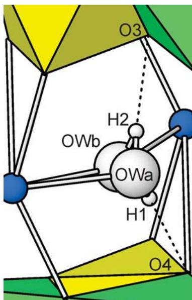
FIG. 4. Bonding of the H<sub>2</sub>O group in andychristyite. Pb–O bonds are shown as sticks and hydrogen bonds as dashed lines. Note that the OWa site is only indicated as being bonded to one Pb site; the other Pb site shown is 3.77 Å from OWa.
