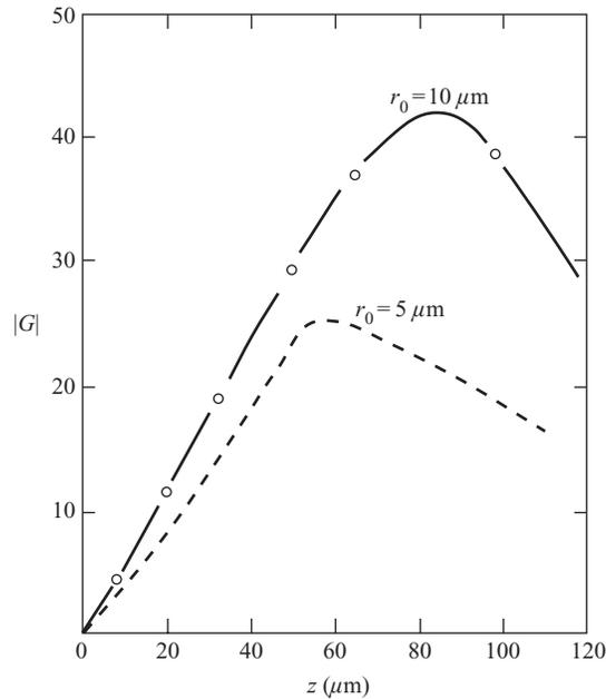
**Figure 2.** Variation of axial gain  $G$  with propagation  $z$  distance.
