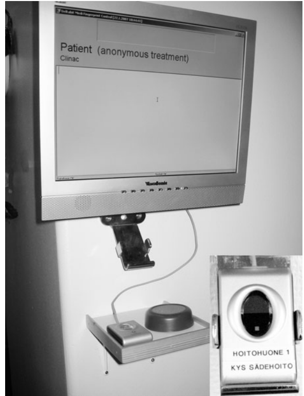
Figure 1. Fingerprint checkpoint reader at the entrance of the treatment room. The reader is enlarged to illustrate the oval-shaped reader window. The sponge for moisturising the finger can be seen.
