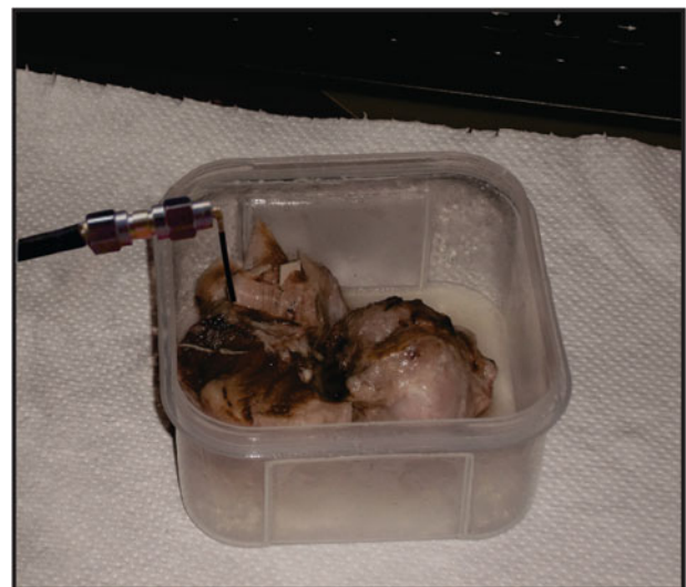
Fig. 4. Dielectric measurement (pork tissue).
