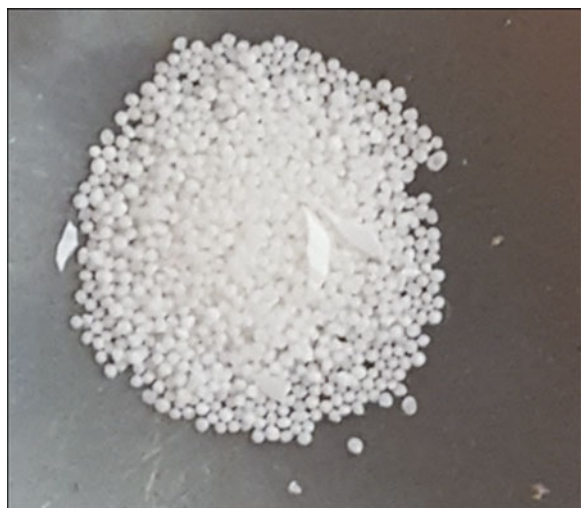
Figure 2. (color online) Microspheres in Linzess ® . Shell pieces were removed before analysis. These microspheres were predominately composed of microcrystalline cellulose I \beta .
