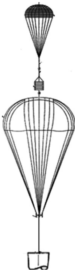
Figure 6. STDS recovery system configuration.
