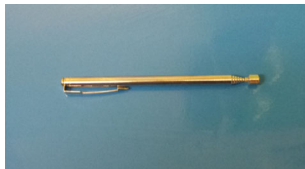
FIG. 1 The magnetic telescopic rod (fully retracted).
