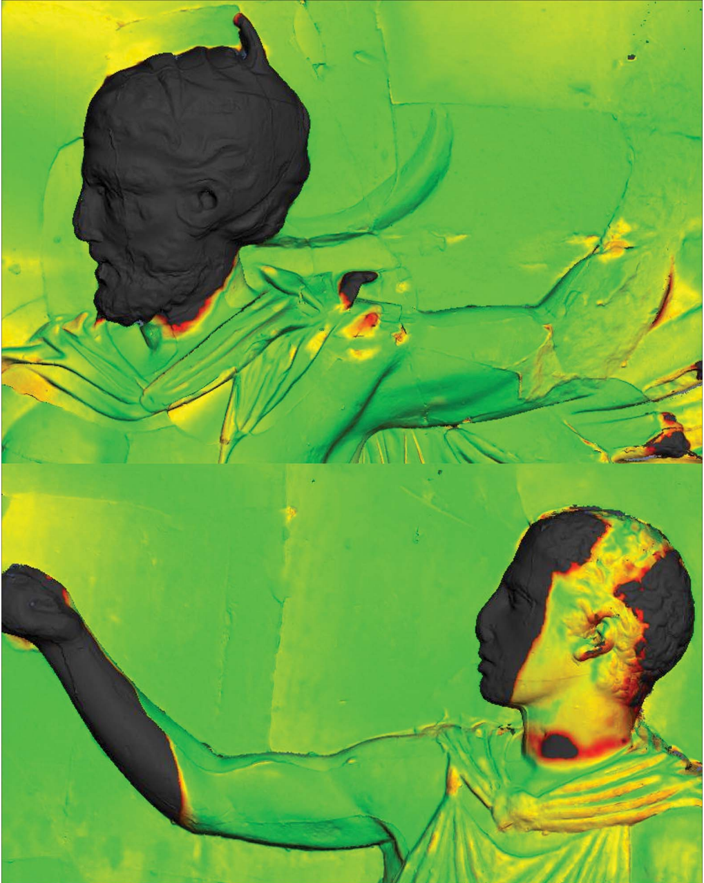
Figure 3. Deviation maps of figure 15 (above: West Frieze VIII) and figure 23 (below: West Frieze XII) at 5mm maximum deviation: greyscale >5mm deviation; red >3mm deviation; yellow >1.5mm deviation; green <1.5mm deviation. Data applied to Elgin casts (images © E. Payne; 3D imaging conducted courtesy of the Trustees of the British Museum).
