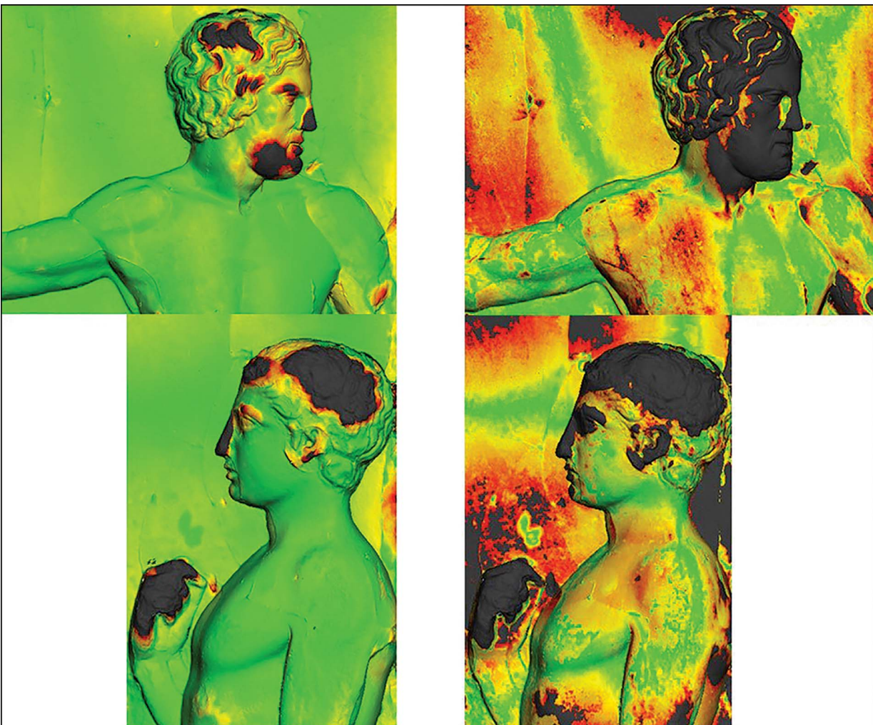
Figure 1. Deviation maps on the left show figures 5 (above) and 6 (below) of West Frieze III at 5mm maximum deviation: greyscale >5mm deviation; red >3mm deviation; yellow >1.5mm deviation; green <1.5mm deviation. Images on the right show the same figures at 1mm maximum deviation: greyscale >1mm; red >0.6 mm; yellow >0.3mm; green <0.3mm. Data applied to Elgin cast (images © E. Payne; 3D imaging conducted courtesy of the Trustees of the British Museum).
