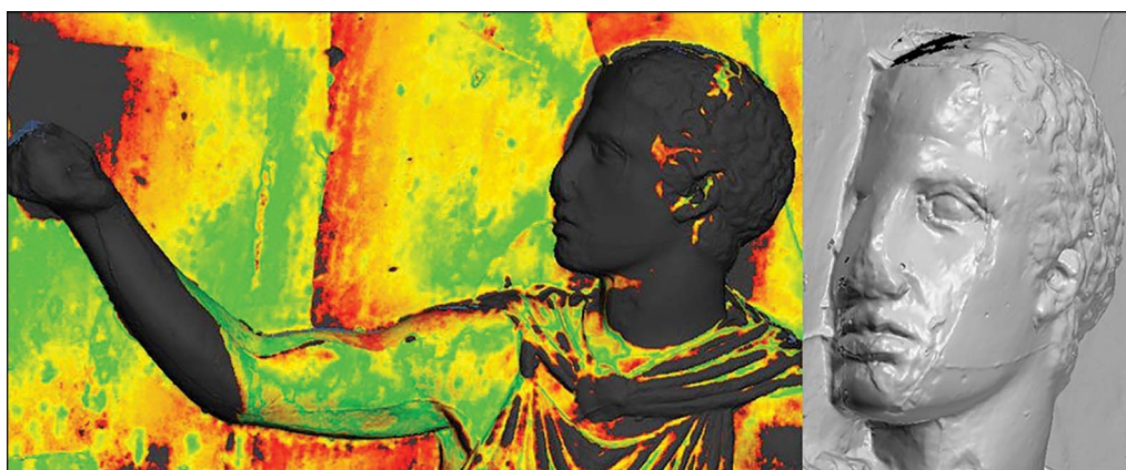
Figure 7. Deviation map of figure 23 (West Frieze XII) at 1mm maximum deviation: greyscale >1mm; red >0.6mm; yellow >0.3mm; green <0.3mm. Data applied to Elgin cast. 3D model with detail of the face to the right (images © E. Payne; 3D imaging conducted courtesy of the Trustees of the British Museum).
