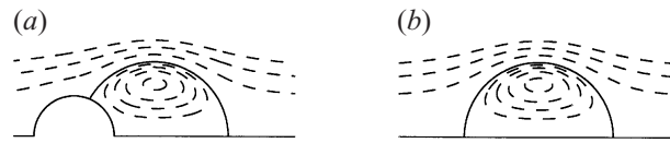
FIGURE 2. Streamlines plot for (a) flow past a sphere with an attached vortex with M = 4 , \omega = 2.2 , and (b) Hill's spherical vortex of radius 1.85, which has the same value of \omega .
