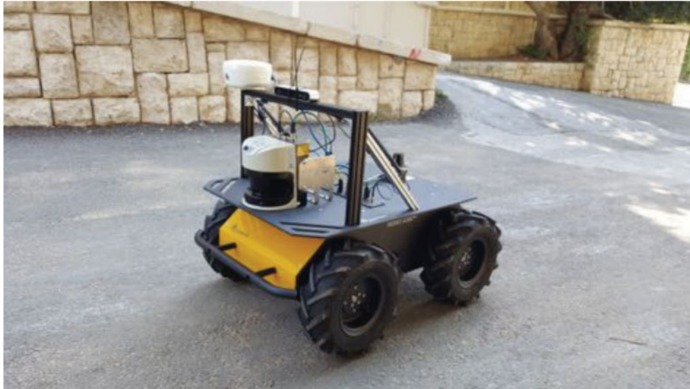
Fig. 4. Deployed sensors and robot. The Zed Stereo Camera is rigidly mounted on top of the Clearpath Husky UGV.
