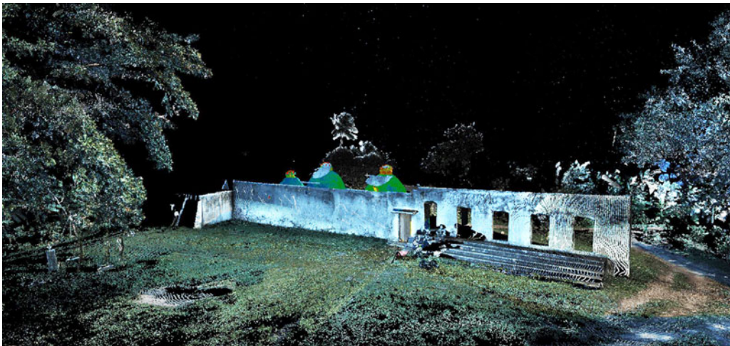
Fig 9. TLS of Kidichi baths showing capture of surrounding topography and vegetation. External point clouds have been draped with photographs. Internal point clouds (bright colours) are displayed using intensity values. Image: Laura Basell.
