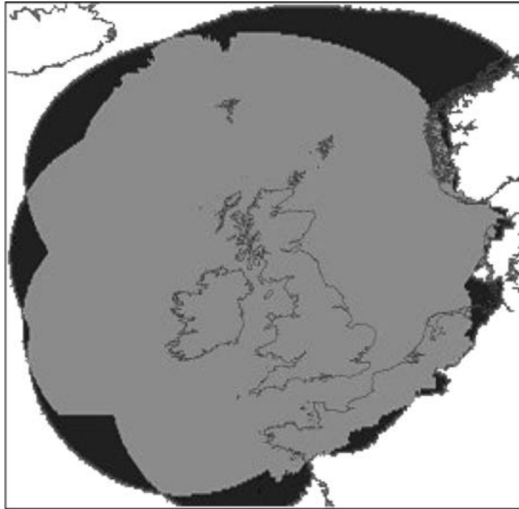
Figure 8. Daytime 3-hour service continuity for the 16 beacons of the UK and Ireland. Light grey=99.97% (critical areas requirement met), Dark grey=99.85% (other areas requirement met).
