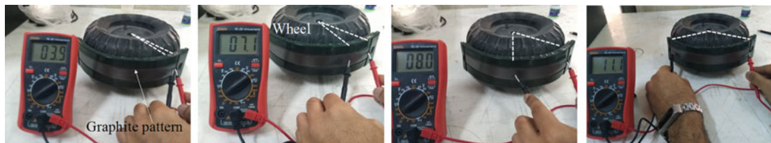
Fig. B2. Sensor test (graphite layer).
