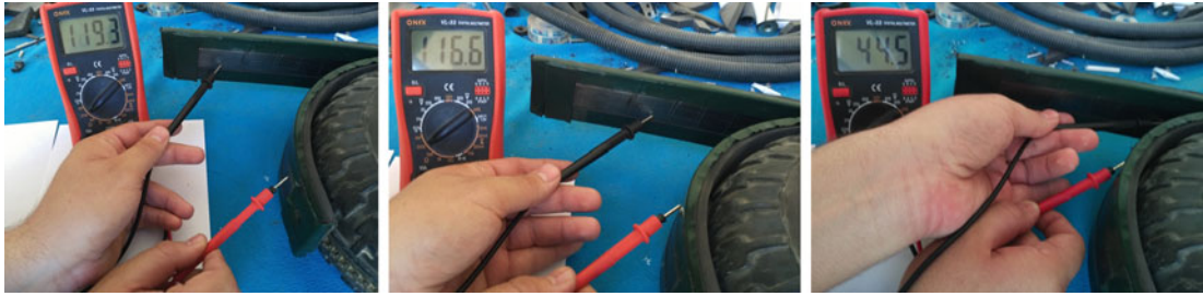
Fig. B3. Sensor test conductive resistive layers.
