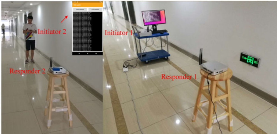
Figure 3. Wi-Fi RTT ranging system.
