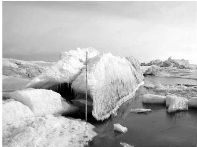
Fig. 10. Evidence that the ice failed through buckling. The stick is \sim 2.4 \text{ m} long marked at 0.2 \text{ m} intervals.
