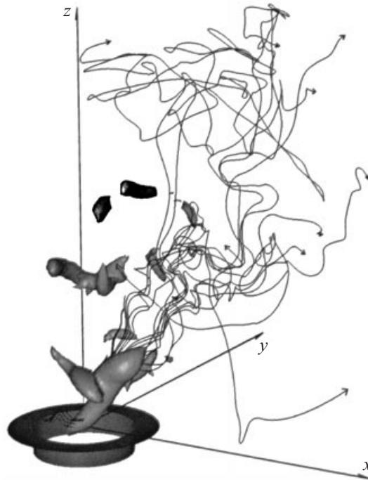
FIGURE 8. Vortex lines through the hanging vortex. Isosurface of pressure at \tilde{p} = -3.6 included to show locations of structures.
