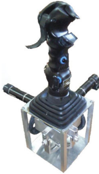
Figure 8. (Colour online) The assembled force-feedback side-stick.
