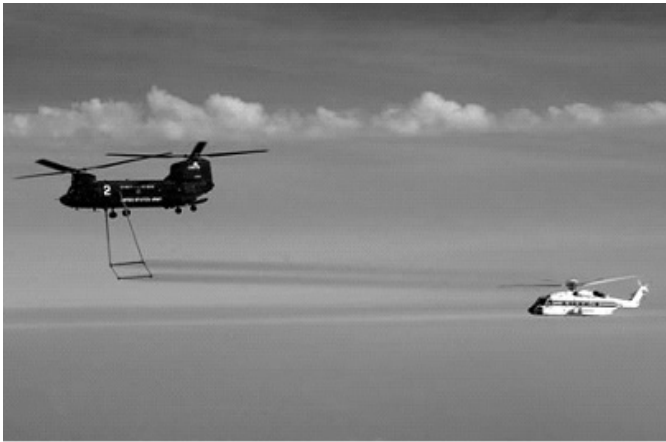
Figure 1. Helicopter Icing Spray System (HISS) (18) .
