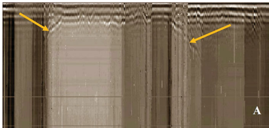
Fig. 5. A GPR traverse to west of KCR with edges of channel arrowed.
