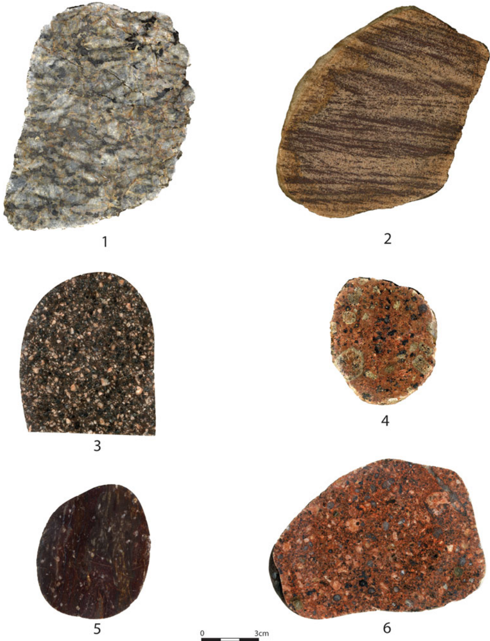
Figure 6. Photographs of polished surfaces of sliced key erratics from the Bruges area. 1. Larvikite (sample HO-28); 2. Kalmarsund sandstone (sample HO-40); 3. Brown Bothnian Sea porphyry (sample HO-18); 4. Rapakivi-type granite (sample HO-63); 5. Dalarna ignimbrite (HO-59); 6. Åland granite-porphyry or Ring quartz porphyry (HO-53).
