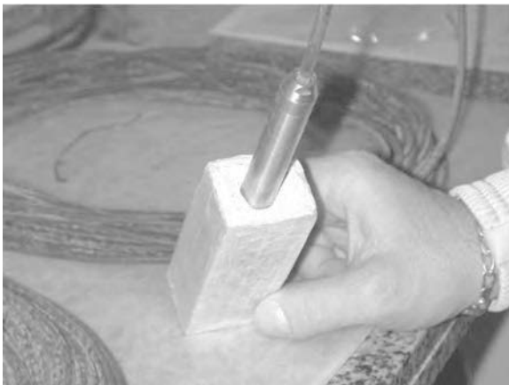
Figure 2. Compacted block of bentonite with a hole drilled for the insertion of the RH sensor.
