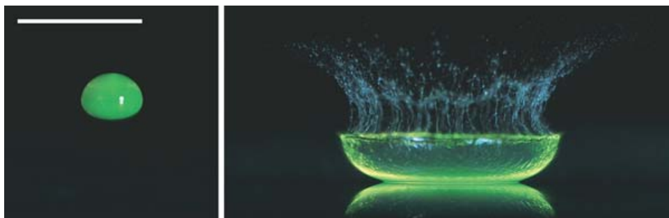
FIGURE 2. The impact of a drop containing Fluorescein dye, for similar impact conditions as in figure 1. The scale bar is 10 mm long.
