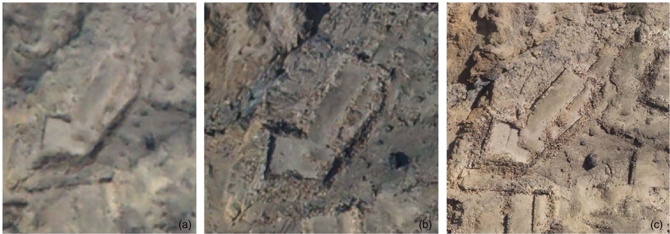
FIGURE 1. (a–c) Differences in resolution and image sharpness due to the height of the camera: (a) 700 m; (b) 470 m; (c) 50 m. In all three cases the camera had a resolution of 24 MP.
