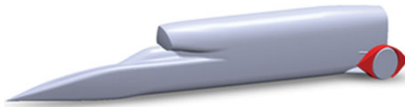
Figure 2. (Colour online) An image of the parametric model of BLOODHOUND SSC with the rear wheel fairing highlighted in red.
