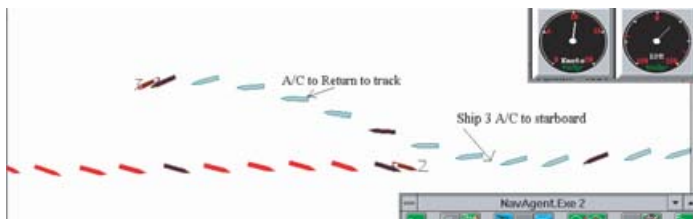
Figure 11. In a current, the head on situation from Figure 7 becomes a crossing situation.
