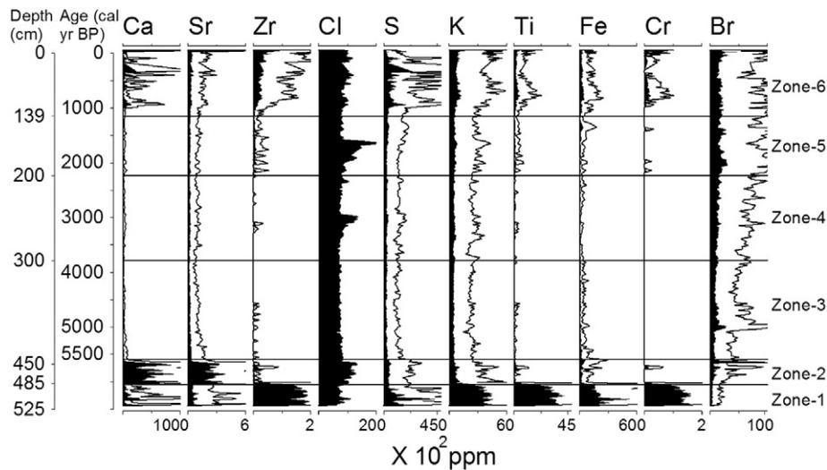
**Figure 5.** XRF results from core SRM-1. Dates on the Y-axis are calibrated yr BP. The black silhouettes represent the actual concentration of the elements, and the transparent curves represent 5X exaggerated values.
